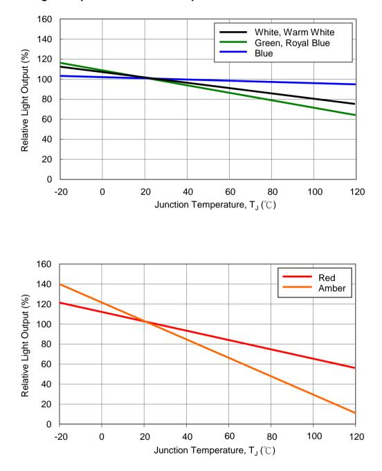
Relative Light Output vs. Junction Temperature at 700mA
