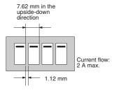
**Note:** The space between each relay required for heat radiation may vary with operating conditions. Contact your OMRON representative for details.
