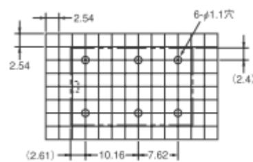
Socket for double-winding latching Models
