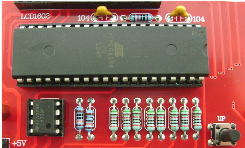
**NOTES:** Please confirm the integrated circuit mounted in correct direction!
