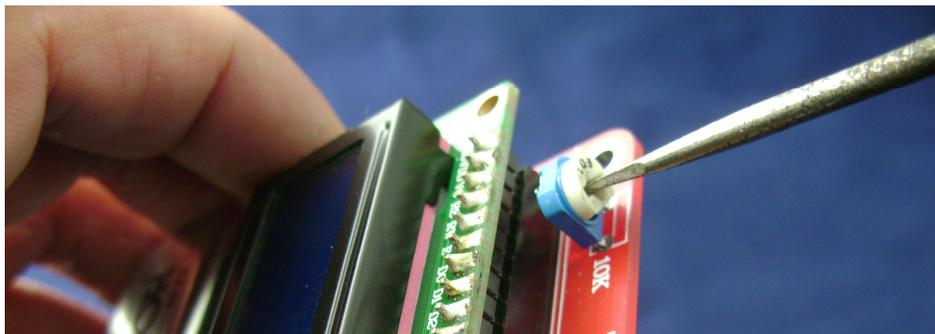
After all the installation, connect the power supply, right adjust the resistance 10K and you will see the character. Adjust the character to clear type.
