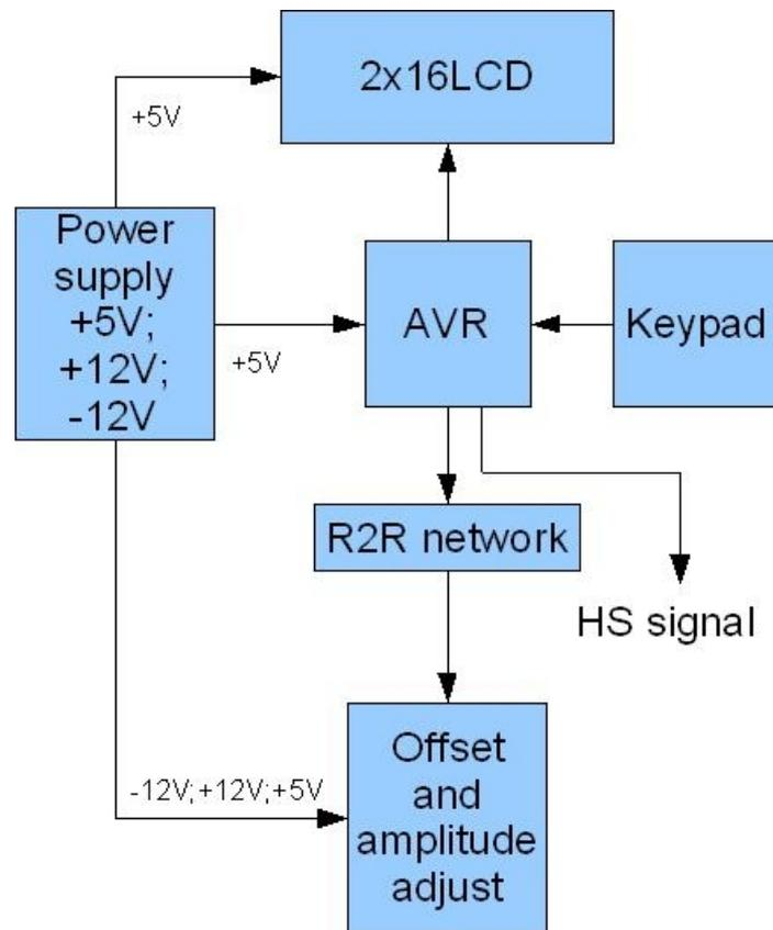
As you can see device requires several voltages: +5V, -12V, +12V, GND. -12V and +12V are used for offset and amplitude control. In this case power supply is constructed by using simple transformer and few voltage regulators, et:7812,7912,7805.
