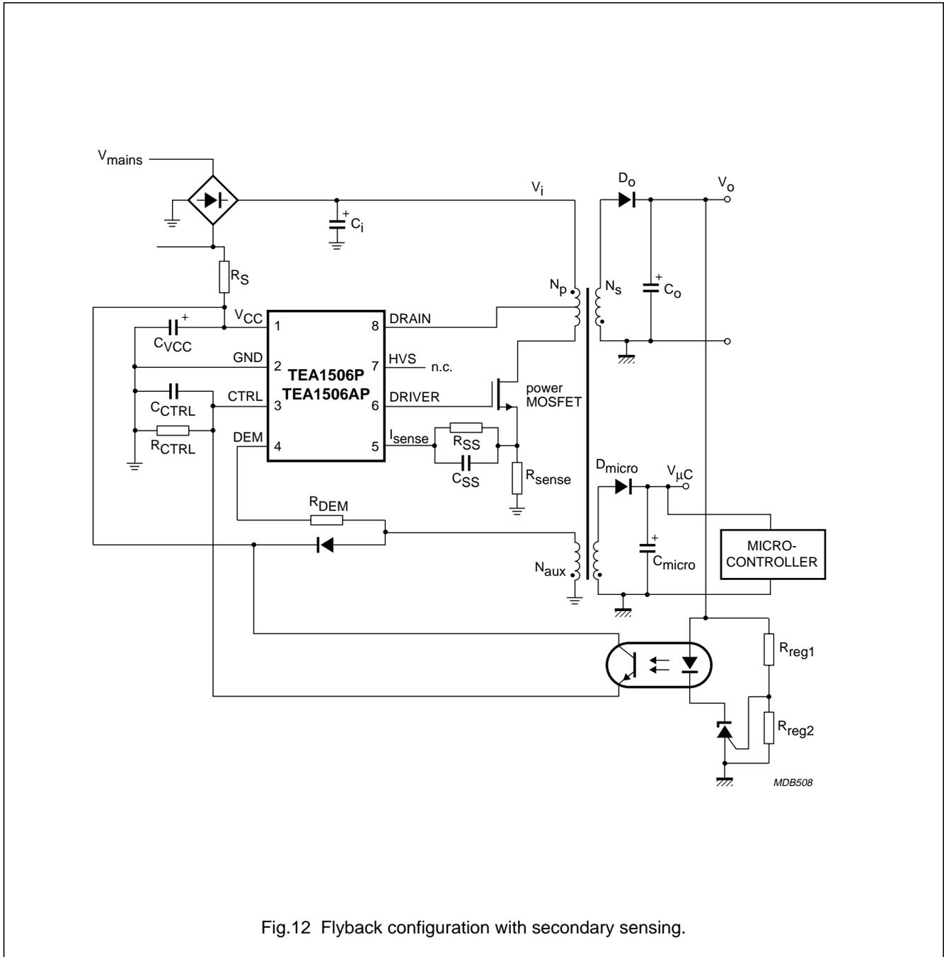
Fig.12 Flyback configuration with secondary sensing.
