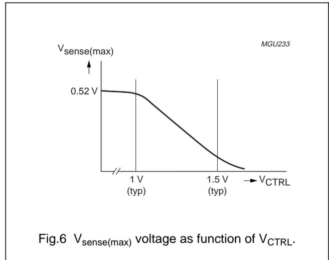
Fig.6  $V_{sense(max)}$  voltage as function of  $V_{CTRL}$ .
