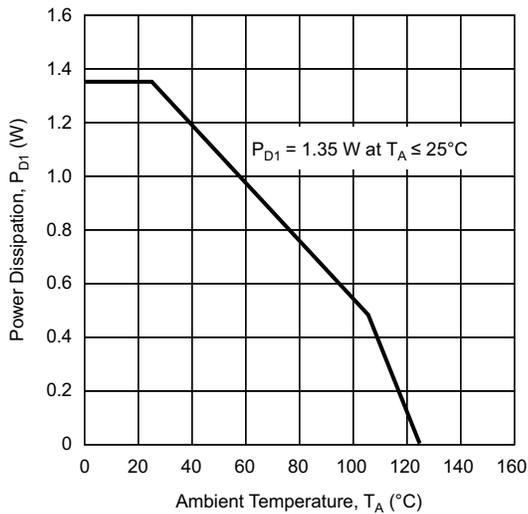
**Figure 6 – MIC Power Dissipation versus Temperature**
