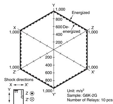
Conditions: Shock is applied in  $\pm X$ ,  $\pm Y$ , and  $\pm Z$  directions three times each with and without energizing the Relays to check the number of contact malfunctions.
