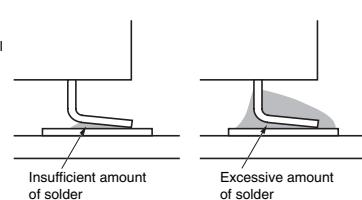
Visually check that the Relay is properly soldered.
