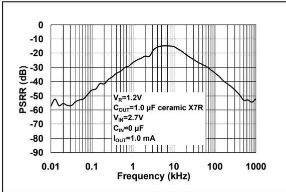
**FIGURE 2-25:** Power Supply Ripple Rejection vs. Frequency.
