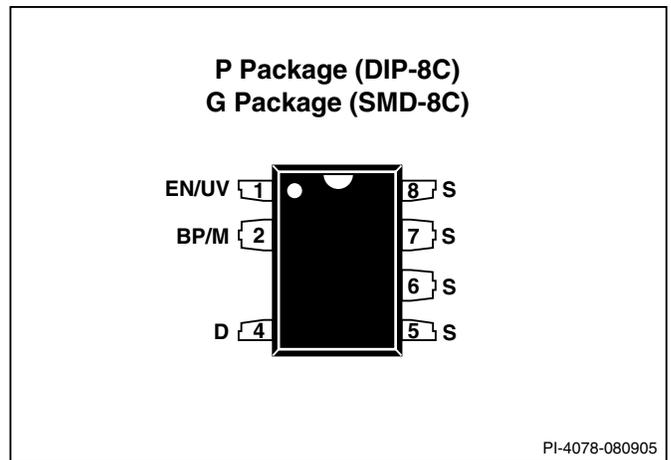
Figure 3. Pin Configuration.
