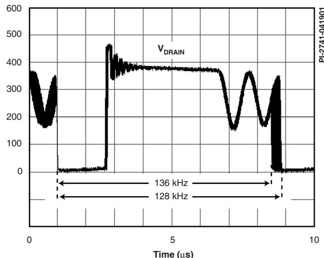
Figure 4. Frequency Jitter.
