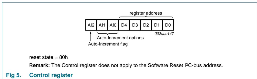
When the Auto-Increment flag is set (AI2 = logic 1), the five low order bits of the Control register are automatically incremented after a read or write. This allows the user to program the registers sequentially. Four different types of Auto-Increment are possible, depending on AI1 and AI0 values.
