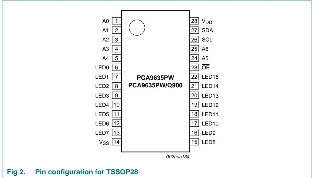
Fig 2. Pin configuration for TSSOP28
