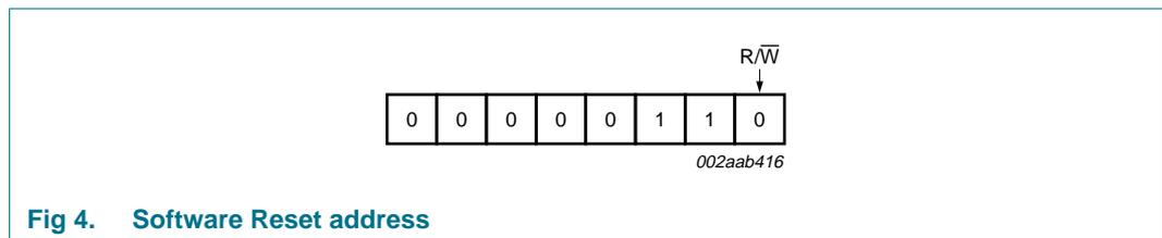
**Remark:** The Software Reset I<sup>2</sup>C-bus address is a reserved address and cannot be used as a regular I<sup>2</sup>C-bus slave address or as an LED All Call or LED Sub Call address.
