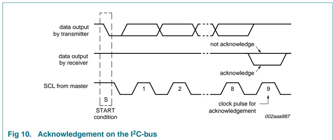
Fig 10. Acknowledgement on the I<sup>2</sup>C-bus
