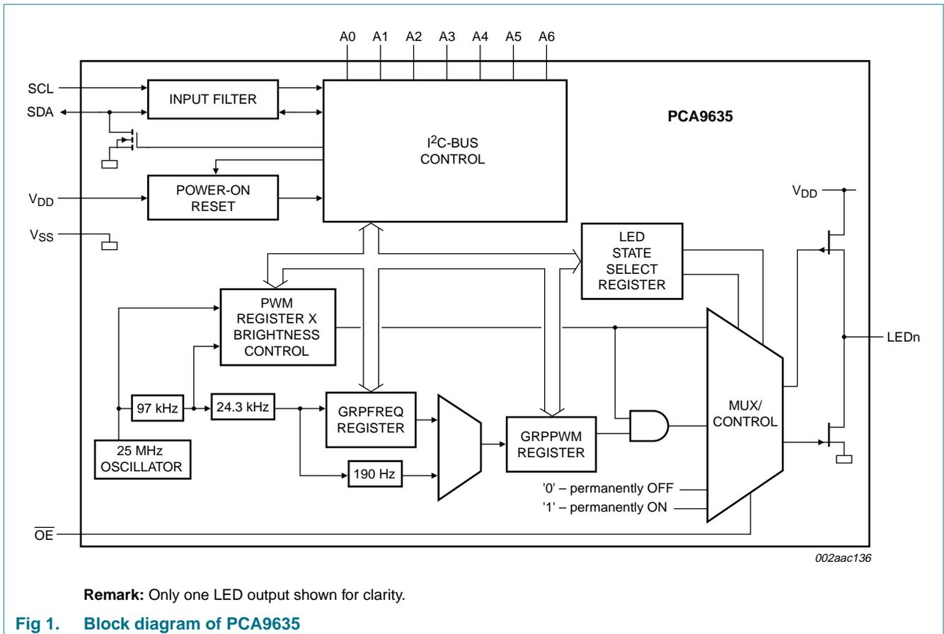
Fig 1. Block diagram of PCA9635
