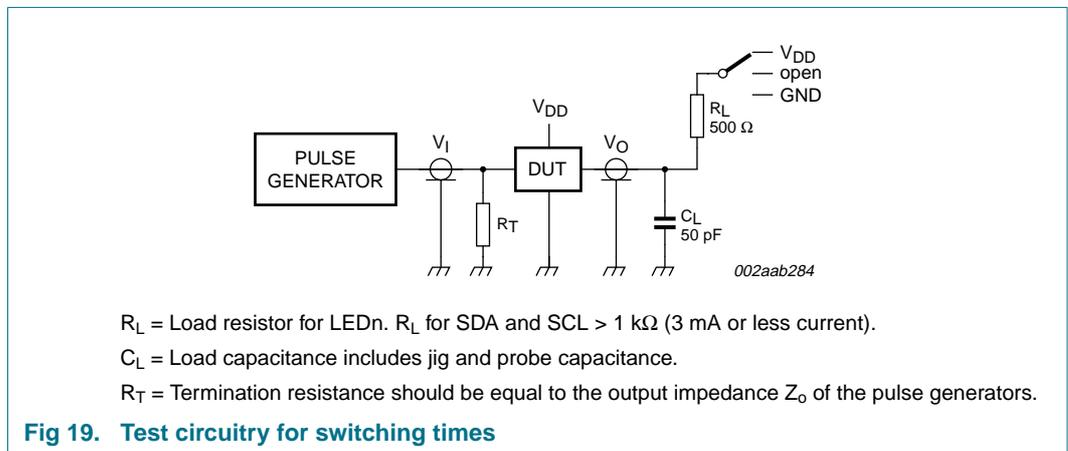
Fig 19. Test circuitry for switching times
