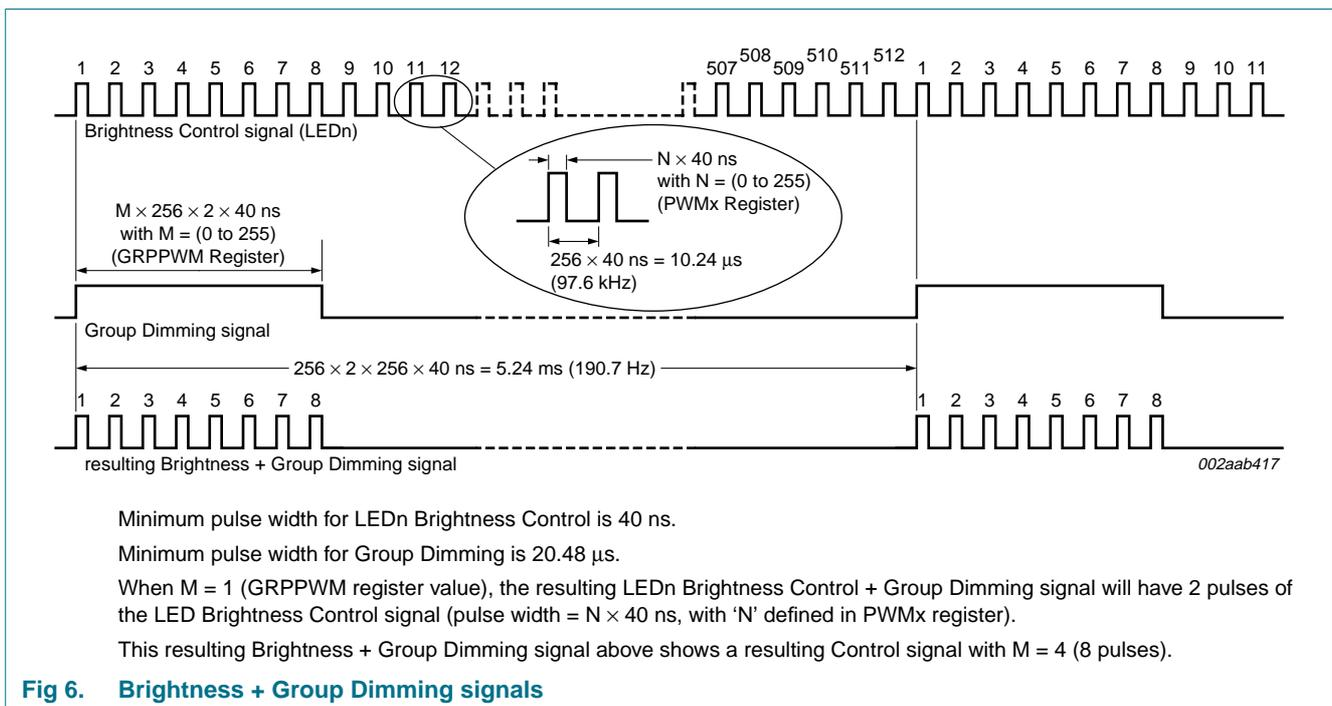
**Fig 6. Brightness + Group Dimming signals**
