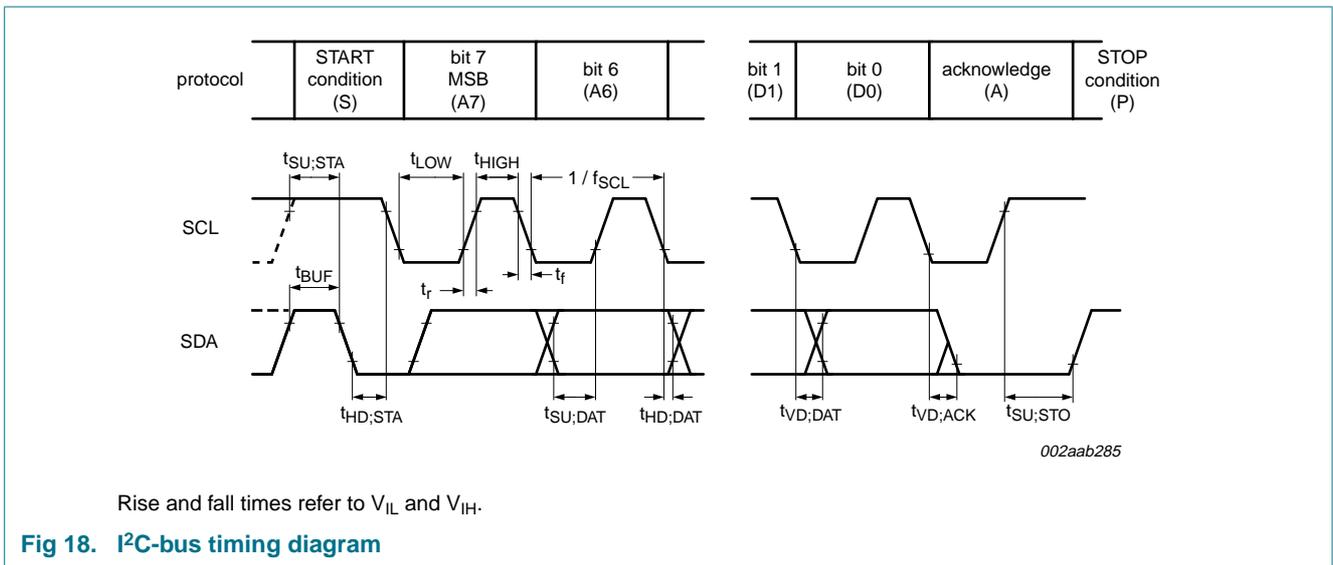
Fig 18. I<sup>2</sup>C-bus timing diagram
