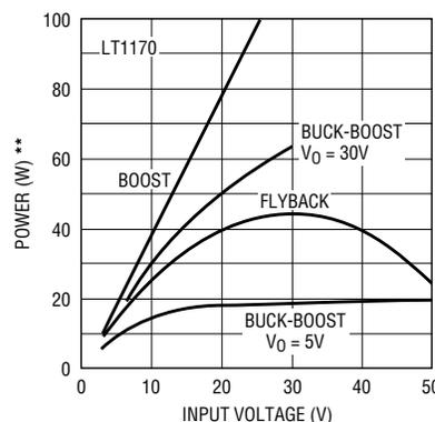
\* ROUGH GUIDE ONLY. BUCK MODE  $P_{OUT} = (5A)(V_{OUT})$ . SPECIAL TOPOLOGIES DELIVER MORE POWER.
