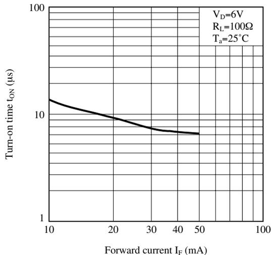
**Fig.9-b Turn-on Time vs. Forward Current (Rank 2)**
