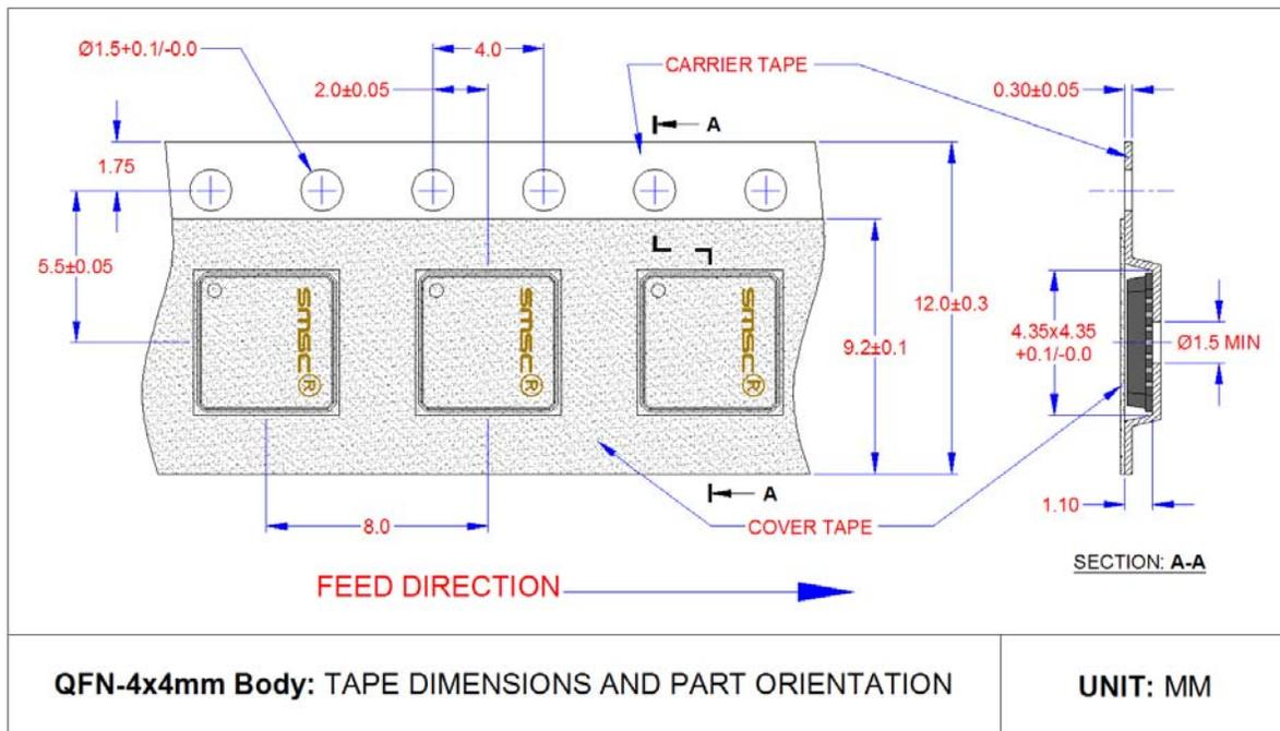
**QFN-4x4mm Body: TAPE DIMENSIONS AND PART ORIENTATION**
