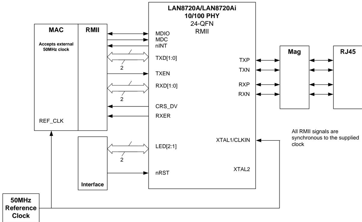
Figure 3.7 External 50MHz clock sources the REF\_CLK
