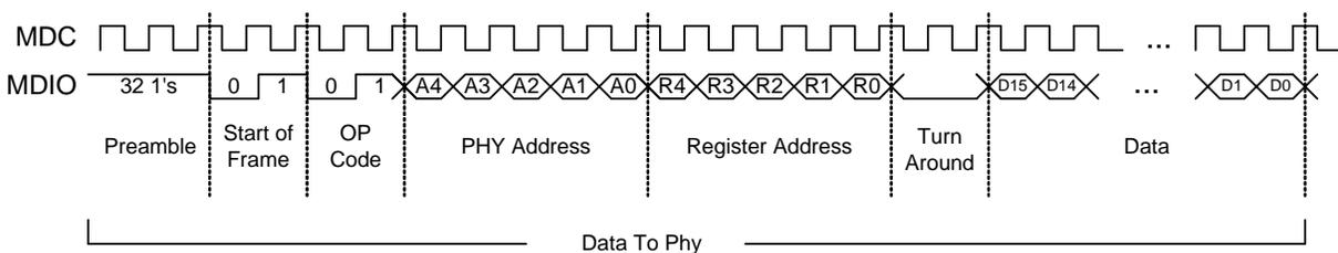
**Figure 3.6 MDIO Timing and Frame Structure - WRITE Cycle**
