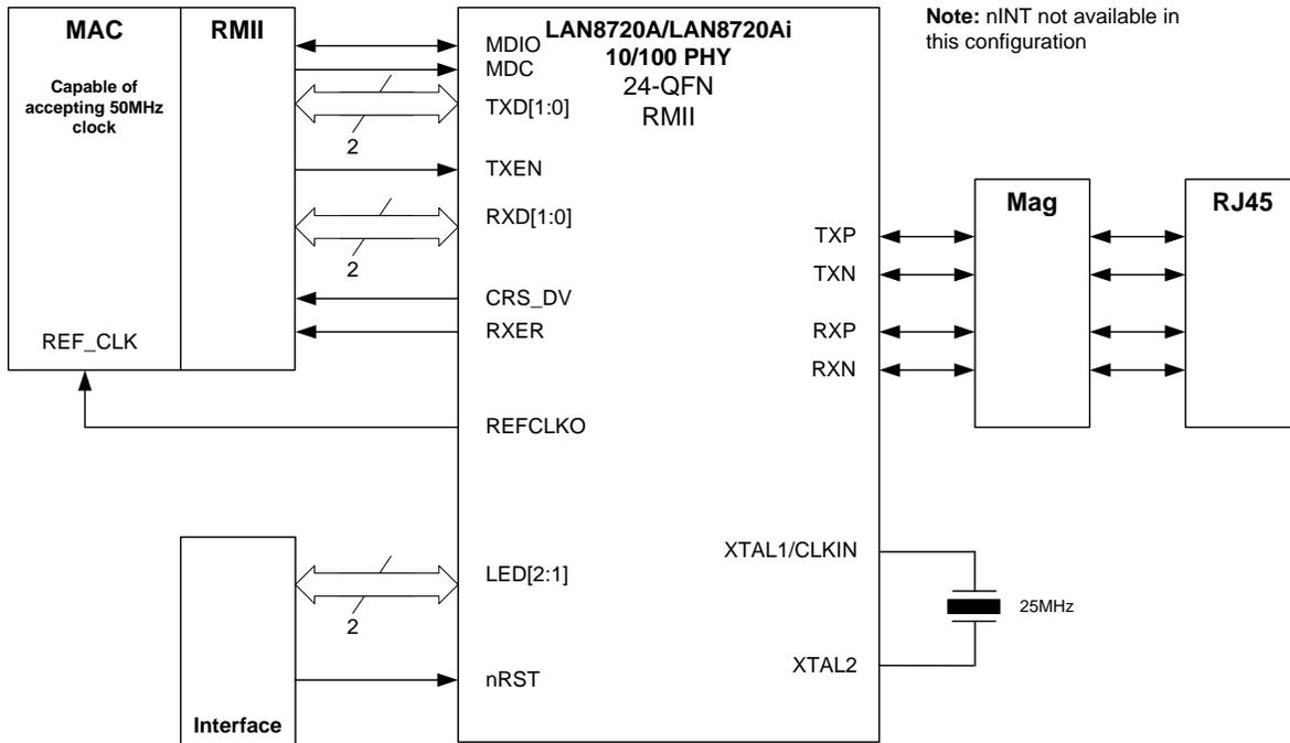
Figure 3.8 Sourcing REF\_CLK from a 25MHz Crystal
