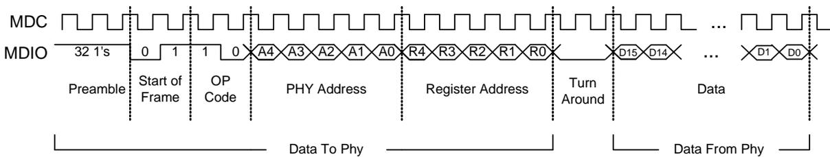
**Figure 3.5 MDIO Timing and Frame Structure - READ Cycle**
