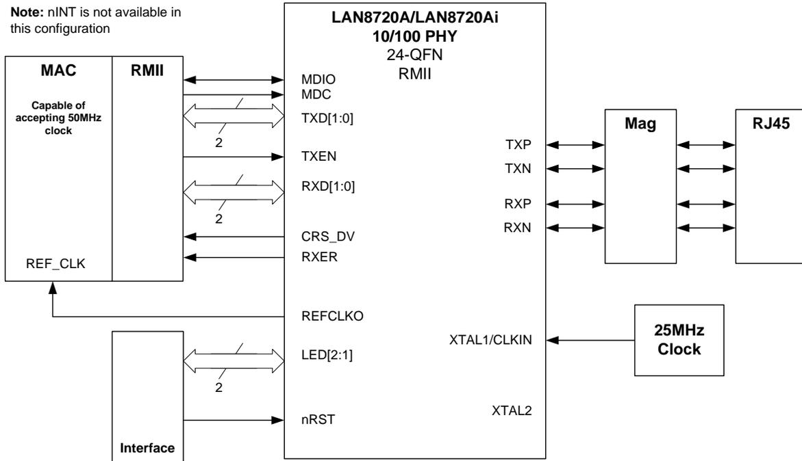
Figure 3.9 Sourcing REF\_CLK from External 25MHz Source
