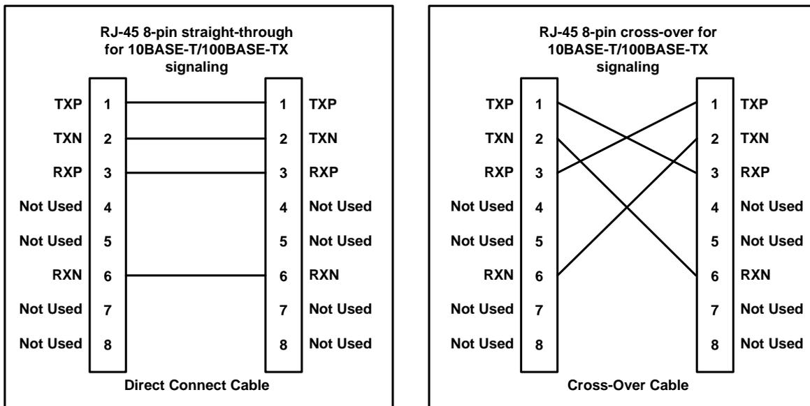
**Figure 3.4 Direct Cable Connection vs. Cross-over Cable Connection**
