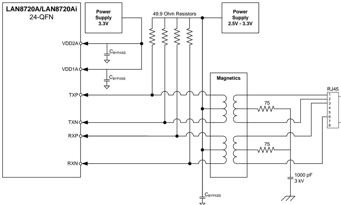
**Figure 3.19 Twisted-Pair Interface Diagram (Dual Power Supplies)**
