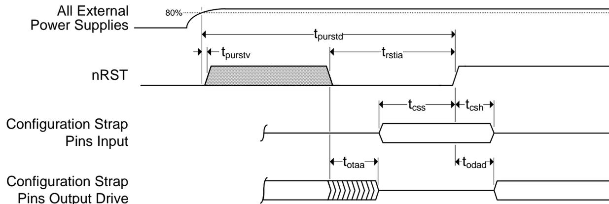
**Figure 5.3 Power-On nRST & Configuration Strap Timing**
