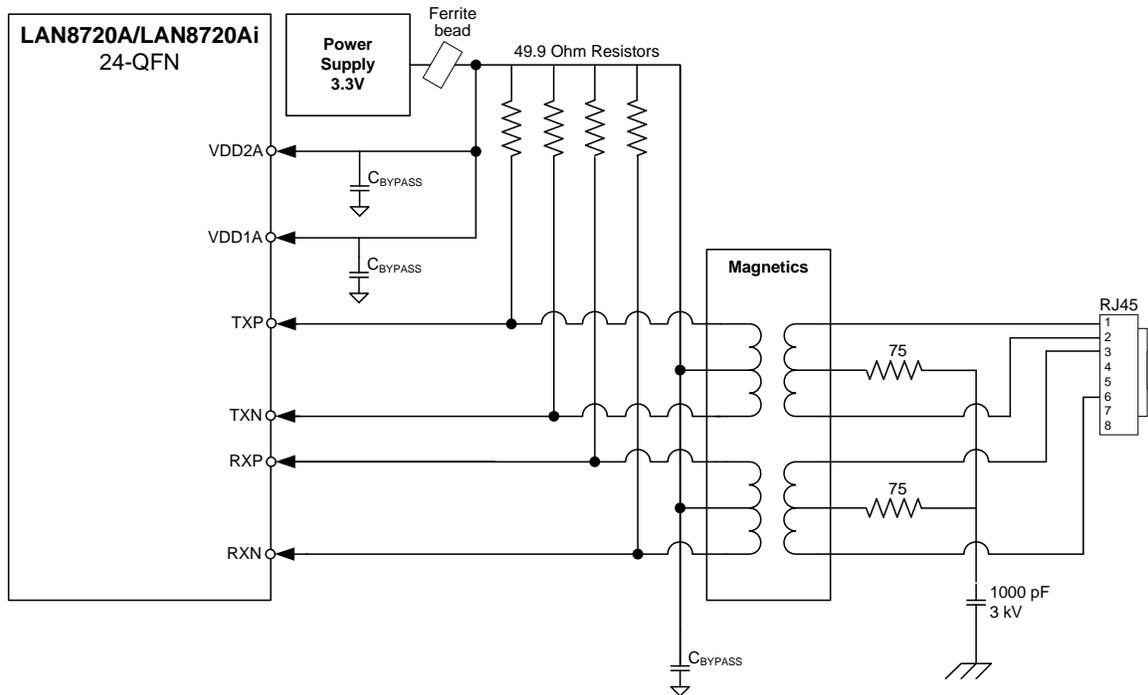
Figure 3.18 Twisted-Pair Interface Diagram (Single Power Supply)
