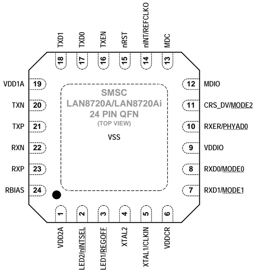
NOTE: Exposed pad (VSS) on bottom of package must be connected to ground
