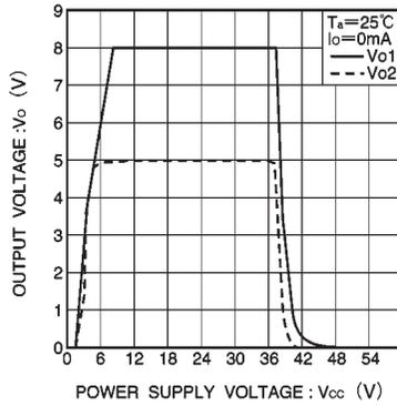
Fig.10 Output voltage characteristics (Typ.)
