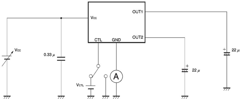
$V_{cc} = 13\text{ V}$ ,  $I_o = 0\text{ mA}$ ,  $V_{CTL} = 5\text{ V}$  when measuring bias current
