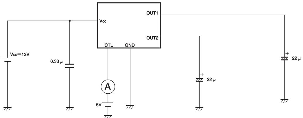
Fig.7 Circuit for measuring input high level current
