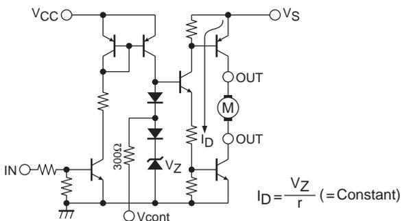
As shown in the left diagram, the Vcont pin outputs the voltage of the band gap Zener  $V_Z + V_F (= 1.93V)$ . In normal use, this pin is left open. The drive current  $I_D$  is varied by the Vcont voltage. However, because the band gap Zener is shared, it functions as a bridge.
