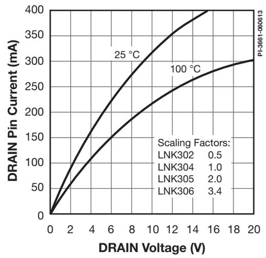
Figure 15. Output Characteristics.
