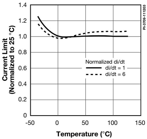
Figure 12. Current Limit vs. Temperature at Normalized di/dt.
