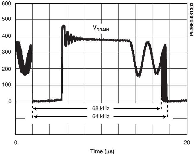
Figure 4. Frequency Jitter.
