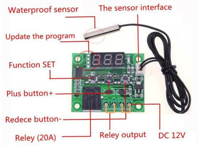
Connect the power supply and equipment, to the controller power supply, as measured temperature is displayed, press the SET button, the display temperature flashes, press "+" "-" to set the desired temperature (hold down the button 5 seconds more quickly lift). After setting press SET to confirm return, then the controller according to the set temperature automatically execute the relay off!
