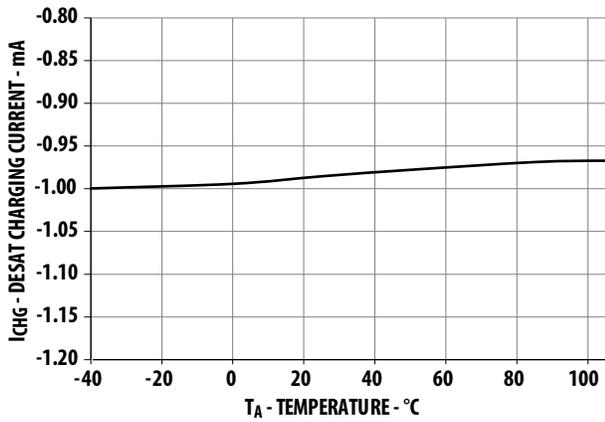
Figure 11. I<sub>CHG</sub> vs. temperature
