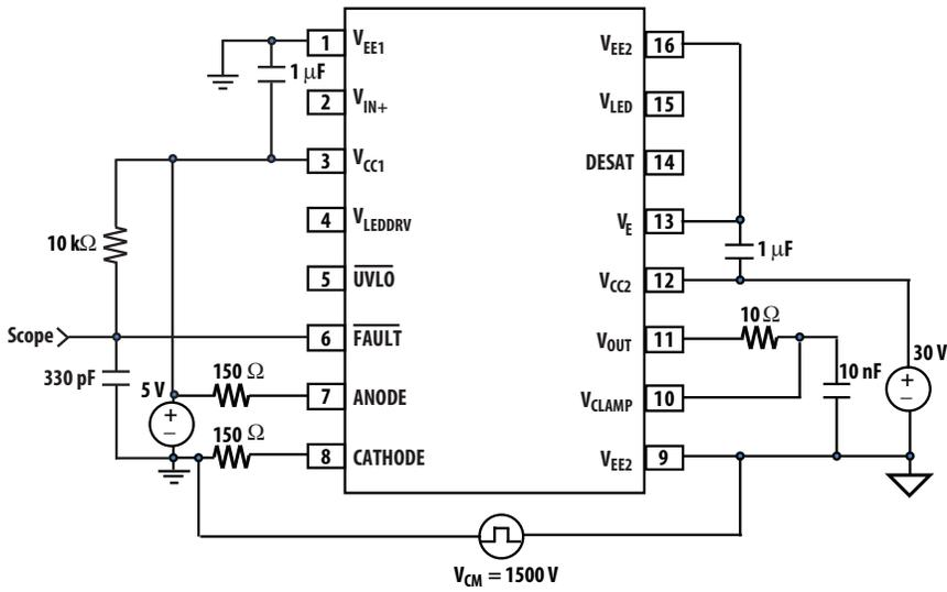
Figure 19. CMR FAULT Low test circuit
