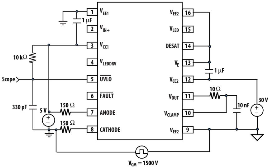
Figure 20. CMR UVLO High test circuit
