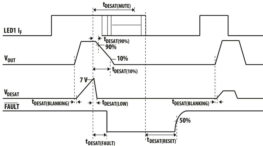
Figure 26. DESAT fault state timing diagram
