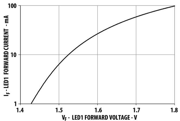
Figure 4. LED1 Input Current vs. forward voltage
