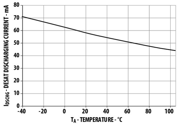
Figure 12. I<sub>DSCHG</sub> vs. temperature
