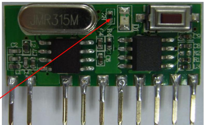
Soldering resistor is Latch Mode
