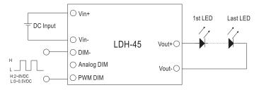
During PWM dimming operation, Io will change with the PWM duty (PWM Signal:  $1K{\sim}10 \text{KHz})$
