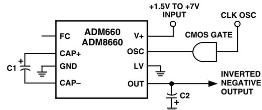
Figure 7. ADM660/ADM8660 External Oscillator
