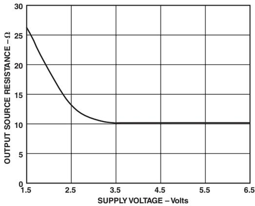
TPC 8. Output Source Resistance vs. Supply Voltage
