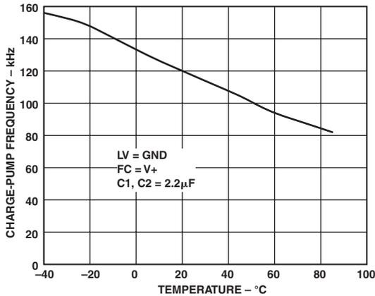
TPC 13. Charge-Pump Frequency vs. Temperature
