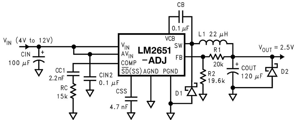
**Figure 16. Schematic for the Typical Board Layout**
