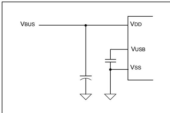
In order to meet the inrush current requirements of the USB 2.0 specifications, the total effective capacitance appearing across VBUS and ground must be no more than 10  $\mu\text{F}$ . If it is more than 10  $\mu\text{F}$ , some kind of inrush limiting is required. For more details on Inrush Current Limiting, search for that subject in the latest "*Universal Serial Bus Specification*".
