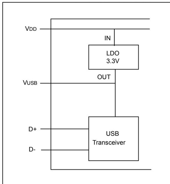
The provided VDD voltage has a direct influence on the voltage levels present on the GPIO and UART Tx/Rx pins. When VDD is 5V, all of these pins will have a logical '1' around 5V with the variations specified in [Section 4.1 "DC Characteristics"](#).
