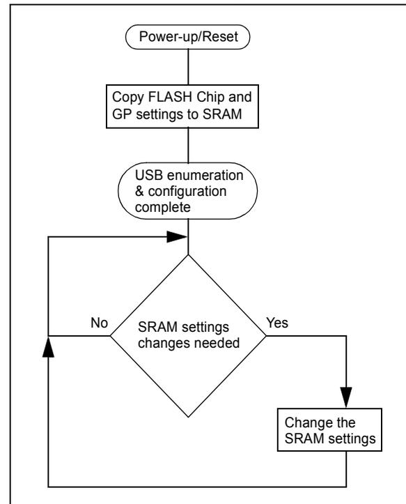
The SRAM settings (GP and partial Chip Settings) can be modified through USB HID commands and they will have an effect on the following device features:
