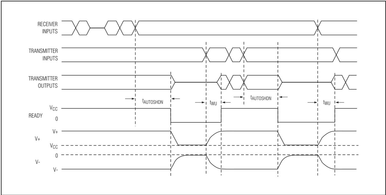
Figure 1. AutoShutdown Plus, and READY Timing Diagram
