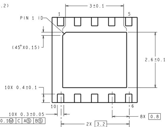
DIMENSIONS ARE IN MILLIMETERS
