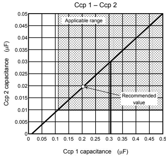
Choose Ccp 1 and Ccp 2 to be combined from the above applicable range. We recommend Ccp 1:Ccp 2 at 10:1 or more. (If our recommended values (Ccp1 = 0.22  $\mu\text{F}$ , Ccp 2 = 0.022  $\mu\text{F}$ ) are used, the drive conditions in the specification sheet are satisfied. (There is no capacitor temperature characteristic as a condition.)
