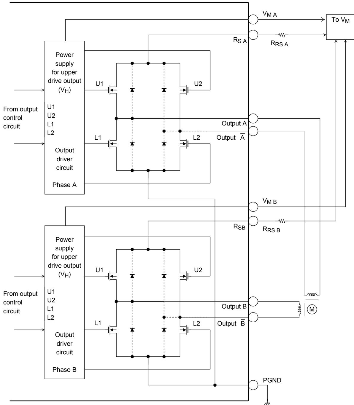
Note: The diode on the dotted line is a body diode.
