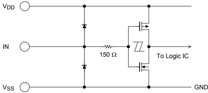
**2. Input circuit (RESET, ENABLE,  $\overline{\text{STANDBY}}$ )**
