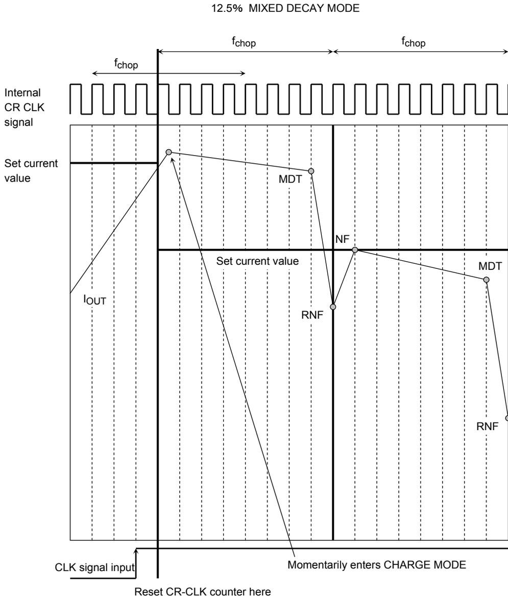
**17. CLK SIGNAL, INTERNAL CR CLK, AND OUTPUT CURRENT waveform
