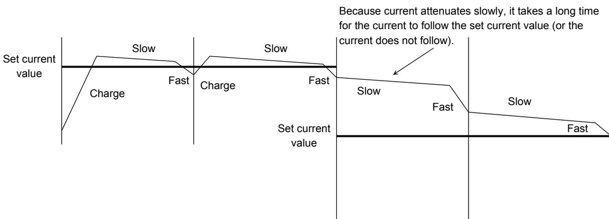
If RNF, current watching point, was the set current value (output current) in the mixed decay mode and in the fast decay mode, there is no charge mode but the slow + fast mode (slow to fast is at MDT) in the next chopping cycle.
