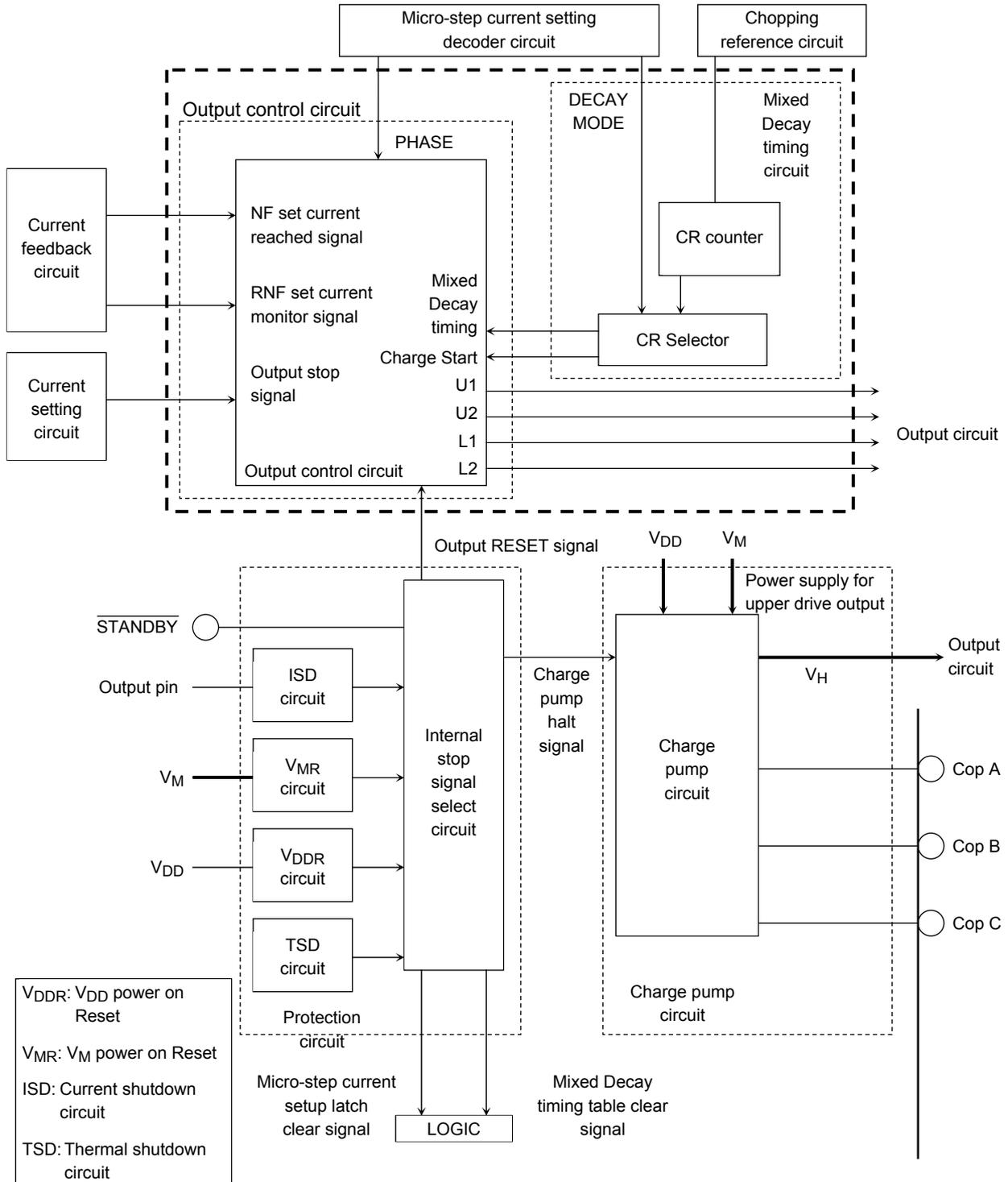
Note: The STANDBY pins are pulled down in the IC by 100-kΩ resistor. When not using the pin, connect it to GND. Otherwise, malfunction may occur.
