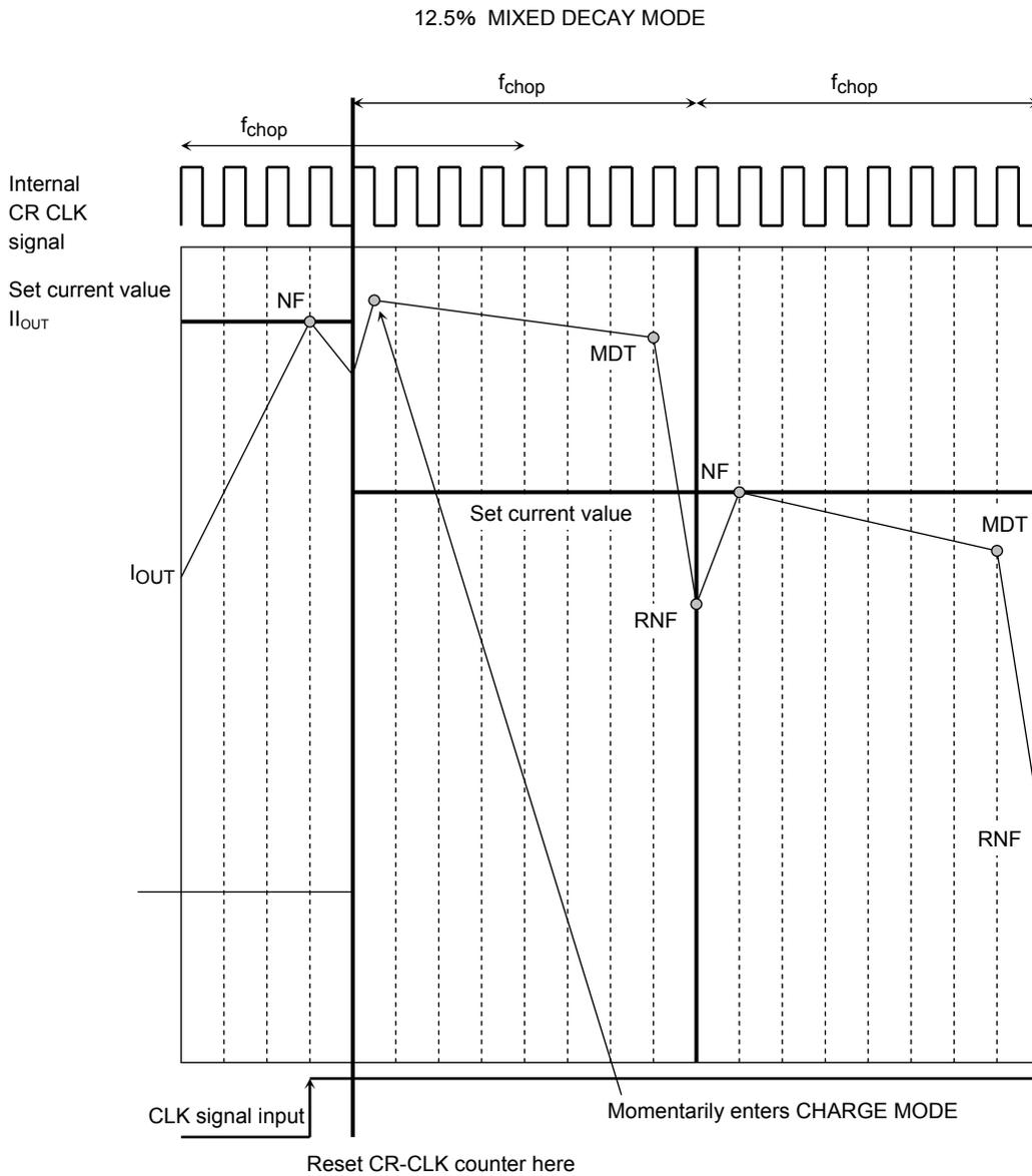
When CLK signal is input, the chopping counter (CR-CLK counter) is forced to reset at the next CR-CLK timing.
