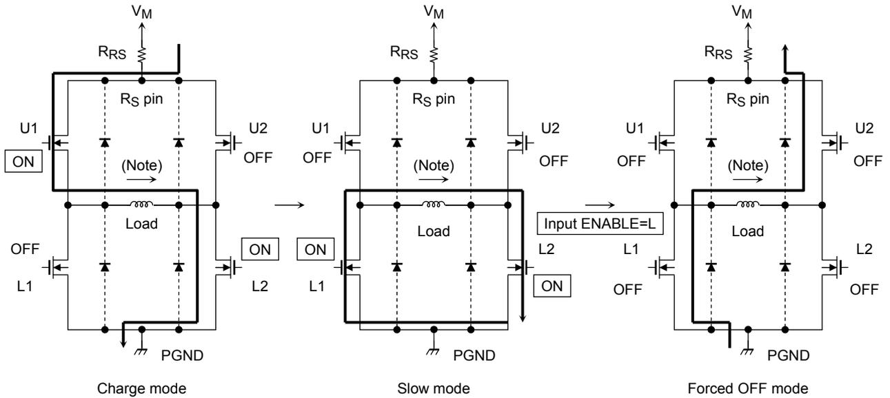
As shown in the figure at above, an output transistor has parasitic diodes.
