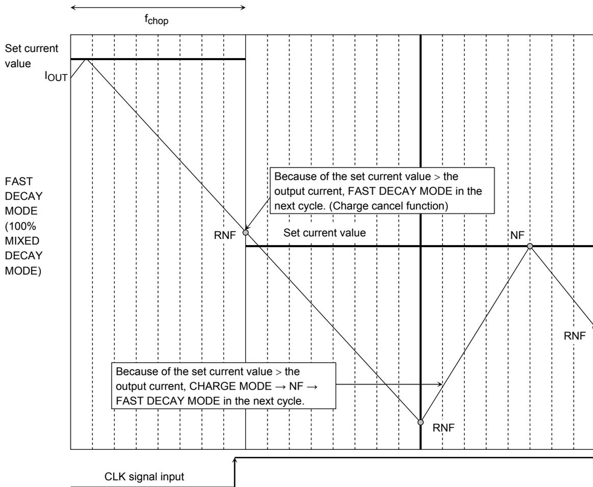
The output current to the motor is in supply voltage mode after the current value set by  $V_{ref}$ ,  $R_{RS}$ , or Torque reached at the set current value.
