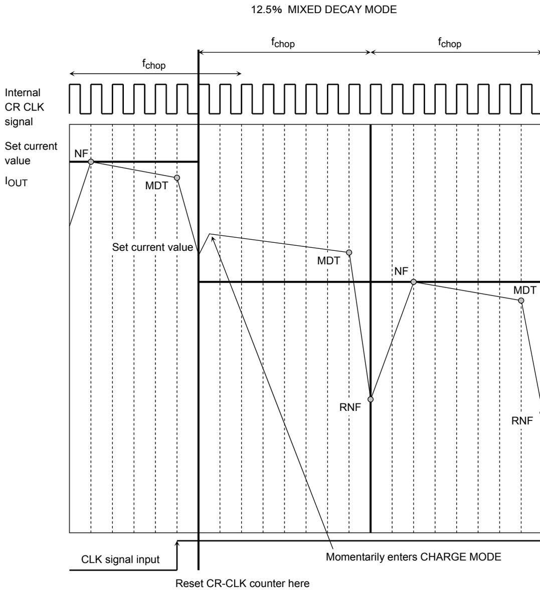
**18. CLK SIGNAL, INTERNAL CR CLK, AND OUTPUT CURRENT waveform (When CLK signal is input in 2 EXCITATION MODE)**
