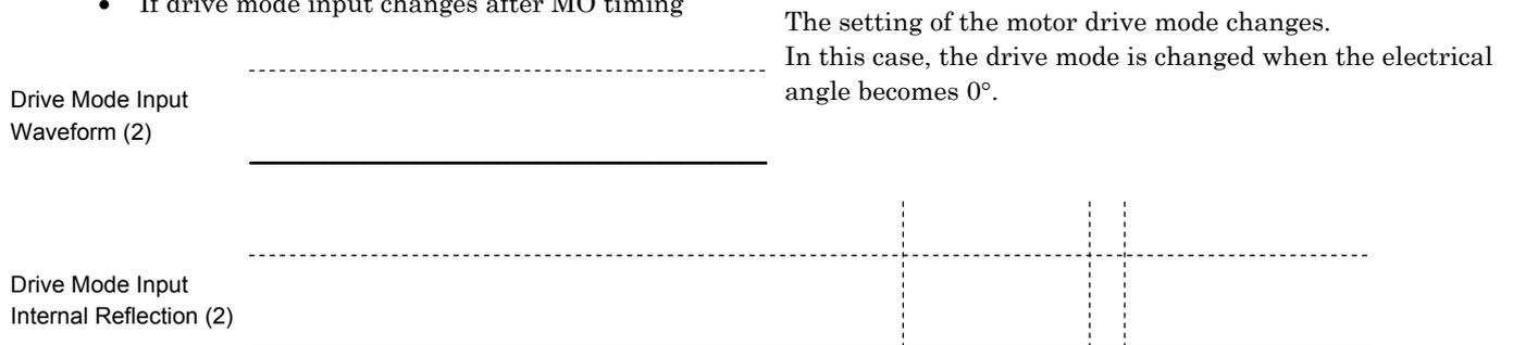
Parallel set signal occurs after the rising edge of CLK, therefore, it is not reflected. The drive mode is changed when the electrical angle becomes 0°.
