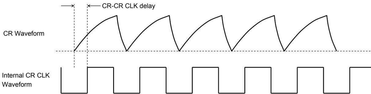
**Figure 2 Timing Waveforms and Names (CR and output)**
