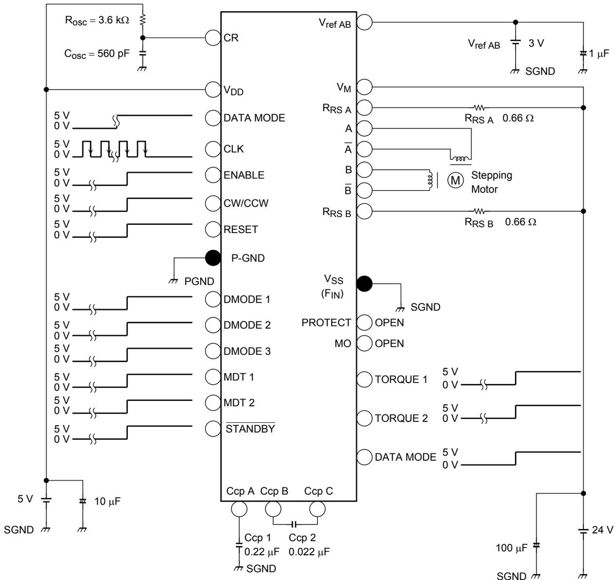
Note: Adding bypass capacitors is recommended.
