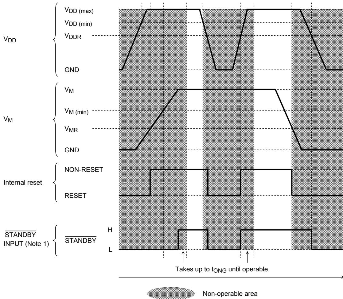
Note 1: If the V<sub>DD</sub> drops to the level of the V<sub>DDR</sub> or below while the specified voltage is input to the V<sub>M</sub> pin, the IC is internally reset.
