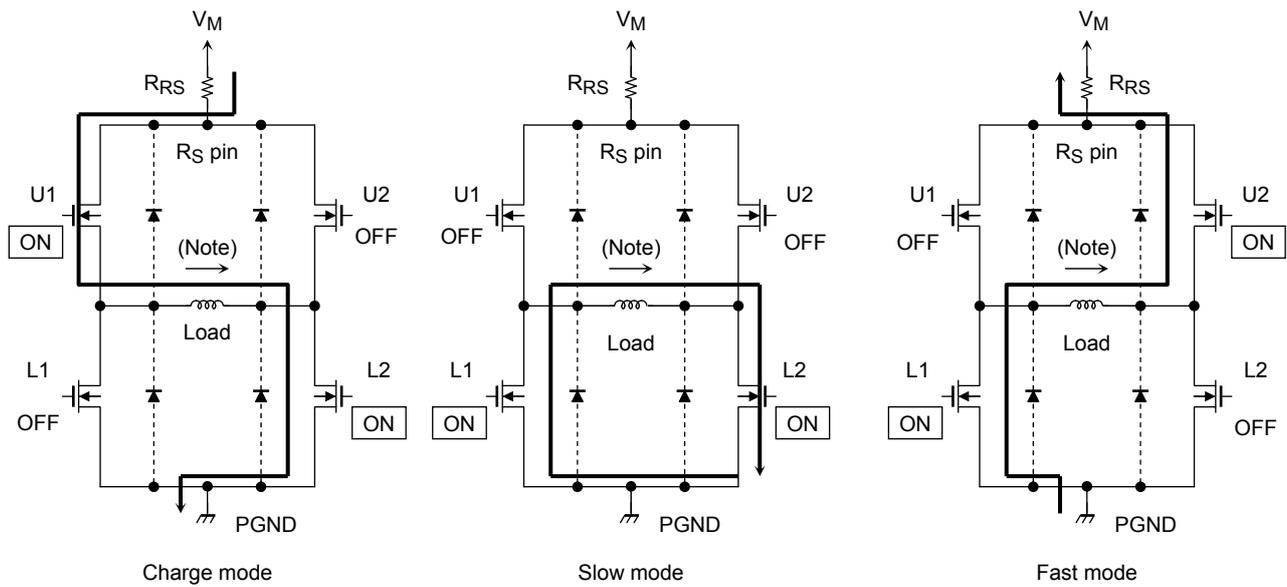
**Output Transistor Operation Functions**
