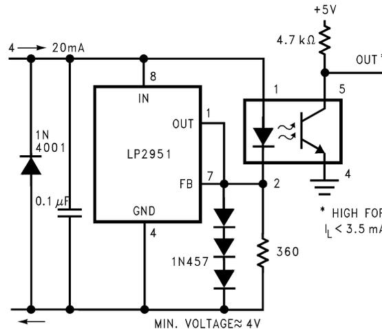
Figure 52. Open Circuit Detector for 4 → 20-mA Current Loop
