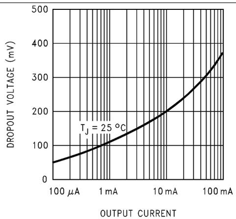
**Figure 12. Dropout Voltage**
