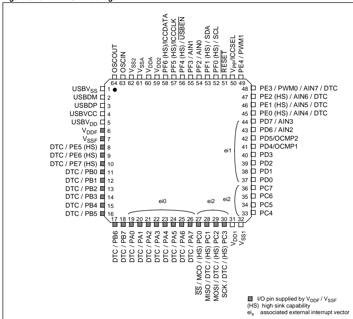
Figure 6. 64-Pin TQFP Package Pinout
