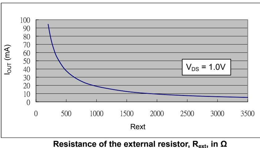
Resistance of the external resistor,  $R_{ext}$ , in  $\Omega$
