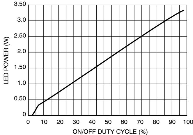
Figure 26. Dimming Characteristic
