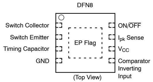
Figure 3. Pin Connections
