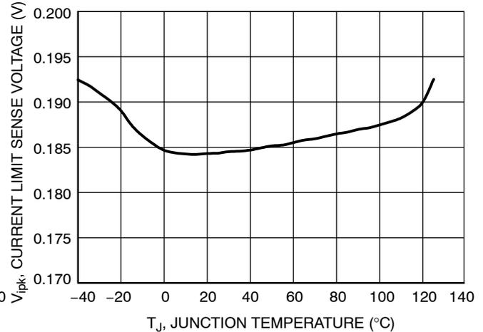
**Figure 10. Current Limit Sense Voltage vs. Temperature**
