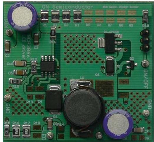
Figure 17. Buck with External Switch Demoboard Photo
