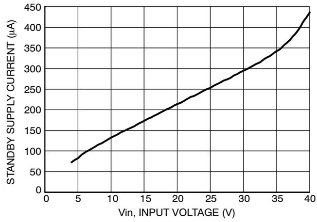
**Figure 11. Standby Supply Current vs. Supply Voltage**
