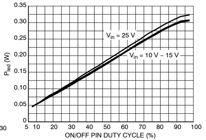
Figure 21. Dimming Characteristic
