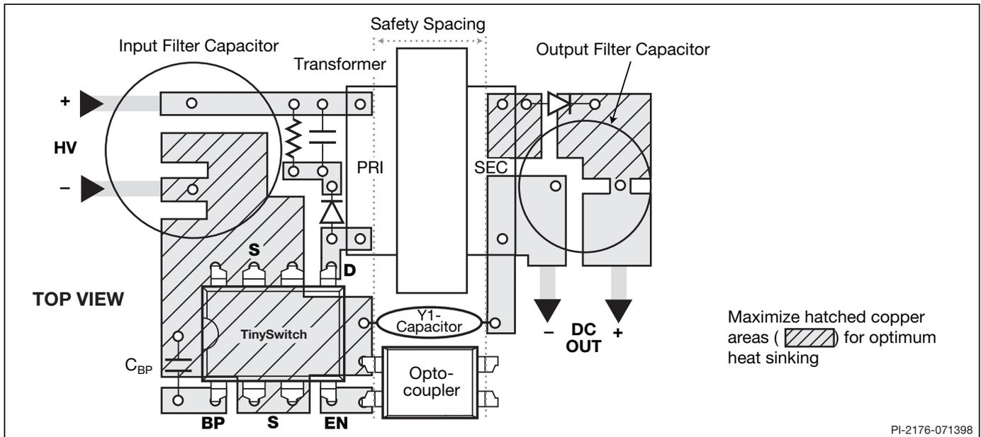
Figure 13. Recommended PC Layout for the TinySwitch.
