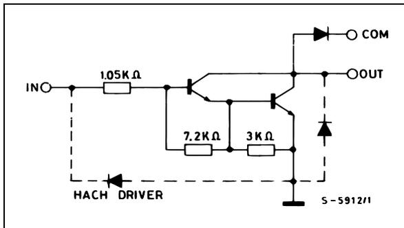
**ULN2801A - ULN2802A - ULN2803A - ULN2804A - ULN2805A**
