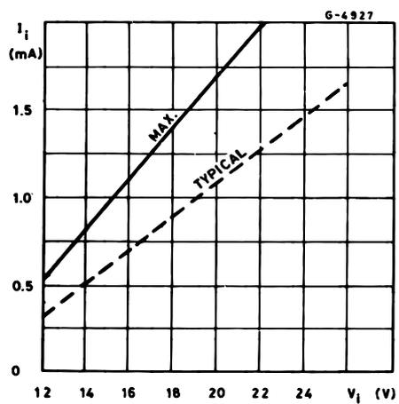
**Figure 14 :** Input Current as a Function of Input Voltage (for ULN2804A)
