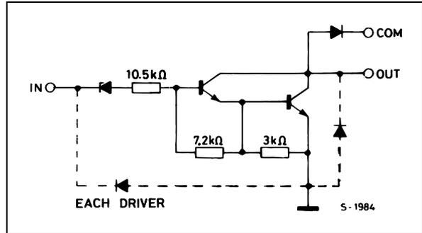
For ULN2803A (each driver for 5 V, TTL/CMOS)
