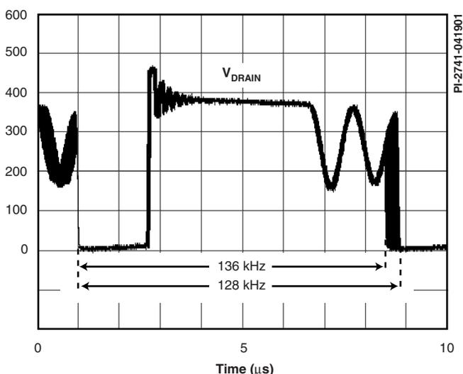
Figure 4. Frequency Jitter.
