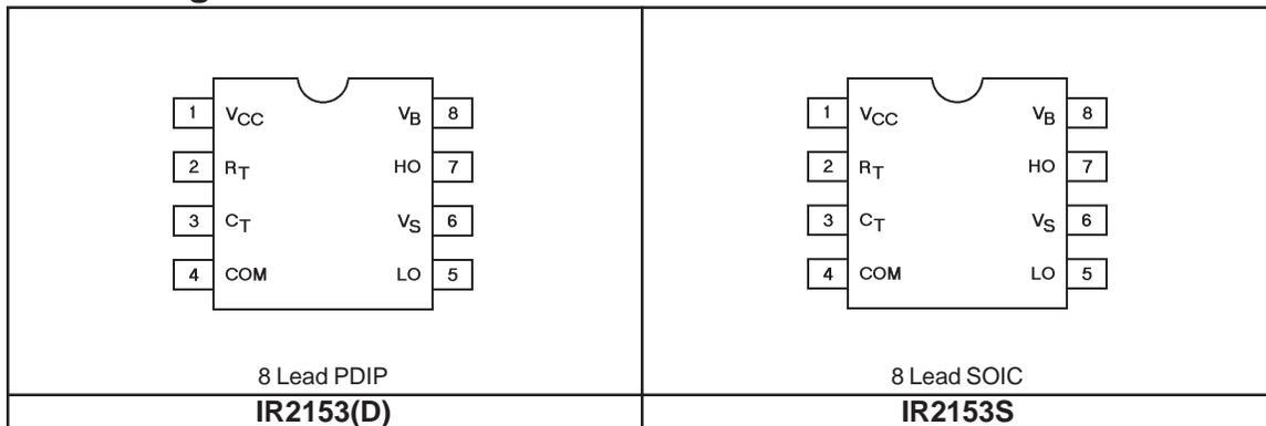
NOTE: The IR2153D is offered in 8 lead PDIP only.
