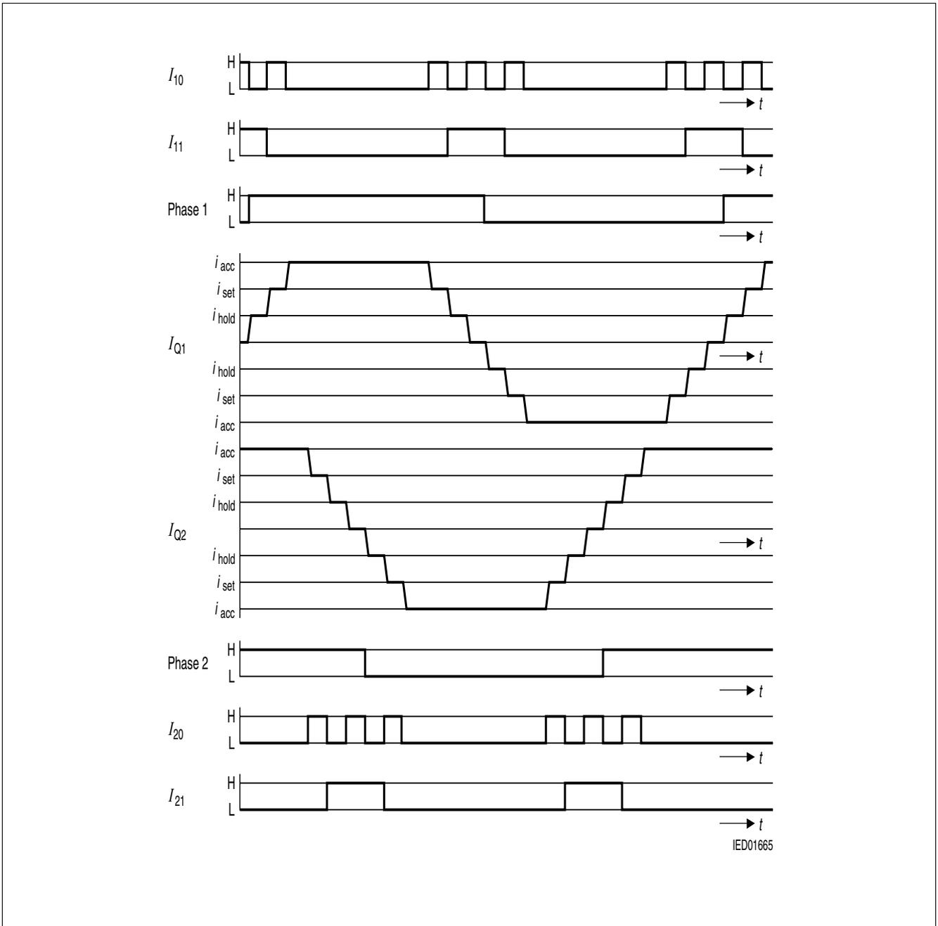
**Figure 8 Mini-Step Operation**
