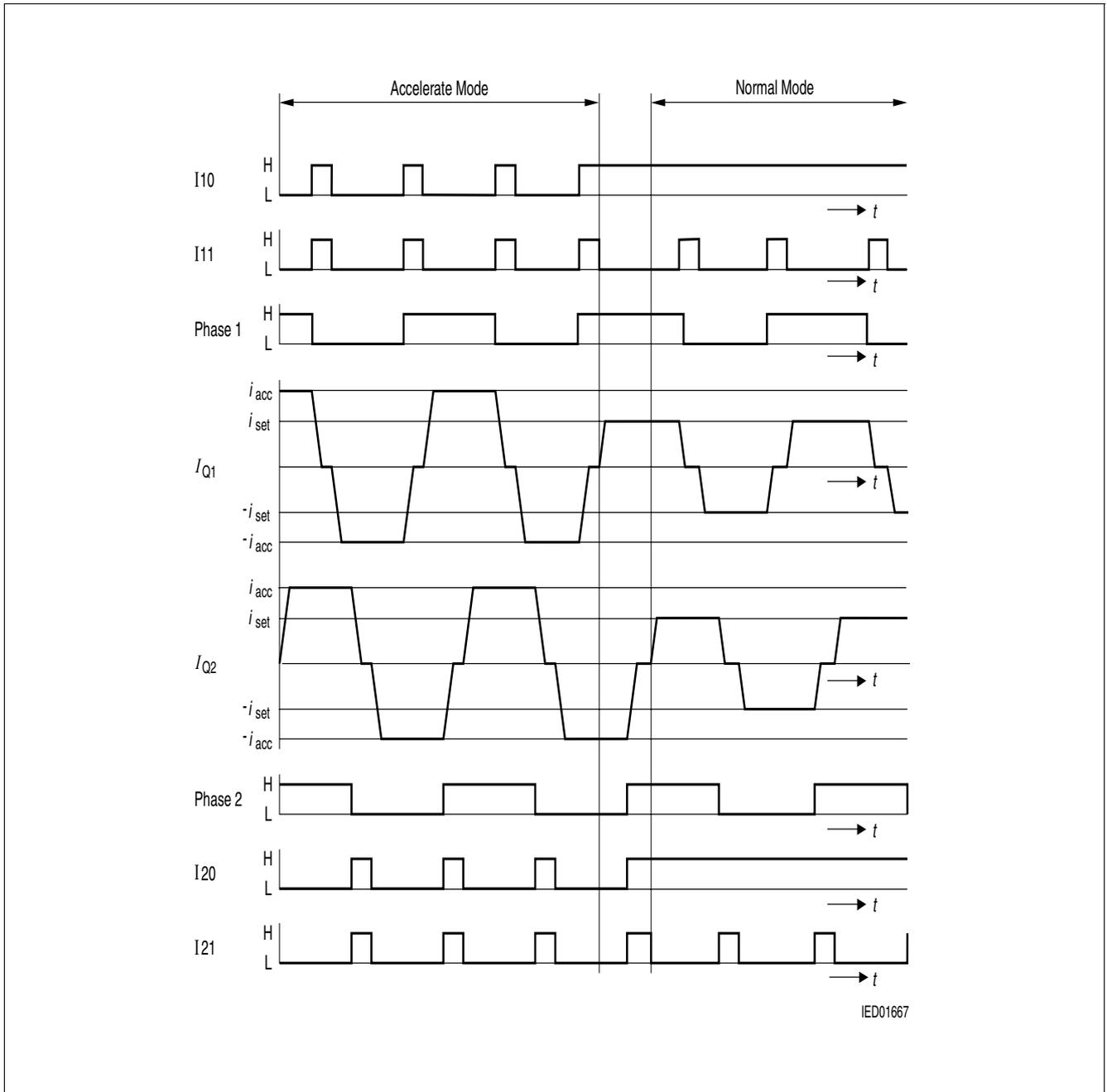
Figure 6 Half-Step Operation
