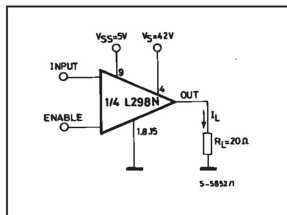
**Figure 3 :** Source Current Delay Times vs. Input or Enable Switching.
