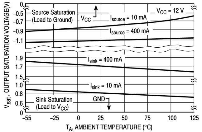
Figure 11. Drive Output Saturation Voltage versus Temperature
