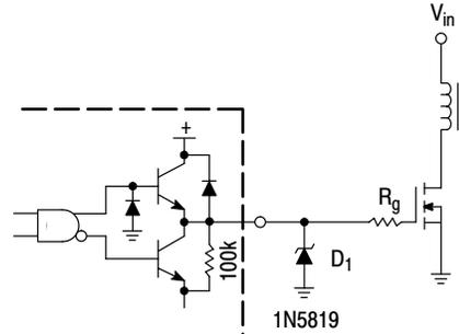
Series gate resistor  $R_g$  may be needed to damp high frequency parasitic oscillations caused by the MOSFET input capacitance and any series wiring inductance in the gate-source circuit.  $R_g$  will decrease the MOSFET switching speed. Schottky diode  $D_1$  can reduce the driver's power dissipation due to excessive ringing, by preventing the output pin from being driven below ground.
