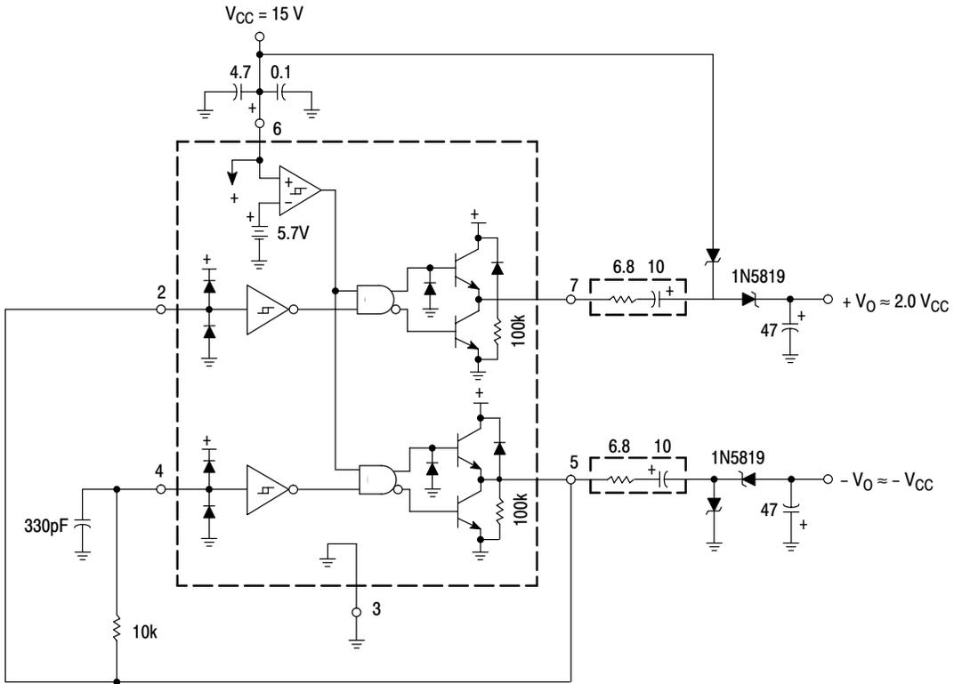
The capacitor's equivalent series resistance limits the Drive Output Current to 1.5 A. An additional series resistor may be required when using tantalum or other low ESR capacitors.
