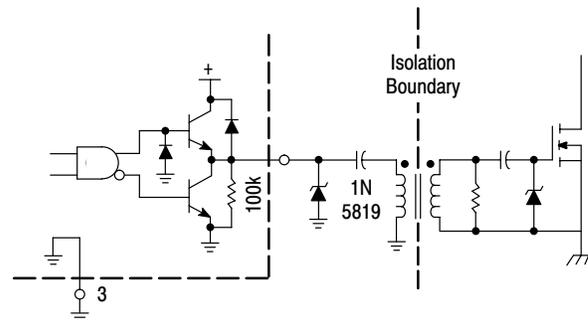
Figure 22. Isolated MOSFET Drive
