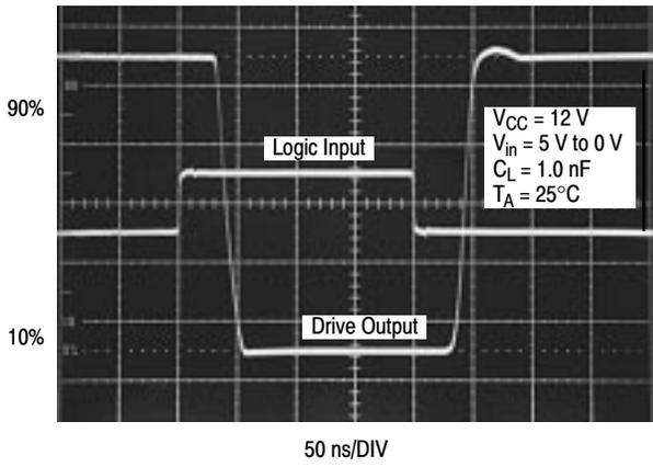
Figure 8. Propagation Delay
